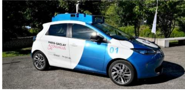
Fig. 1: The autonomous vehicle prototype developed by Groupe RENAULT for EVAPS project. The most evident sensor is the Velodyne UltraPuck LiDAR on top.
